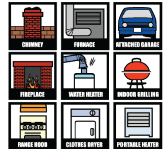
POTENTIAL SOURCES OF CARBON MONOXIDE IN THE HOME
